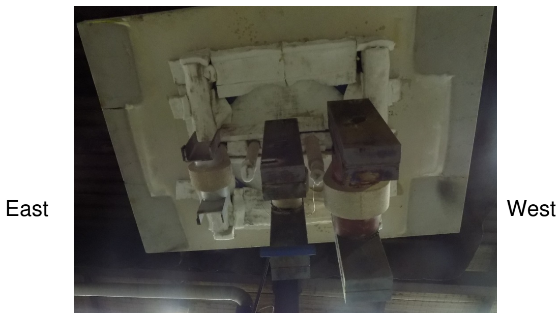
Figure A5.2: Exposed face (bottom view) of specimen before commencement of the fire-resistance test
