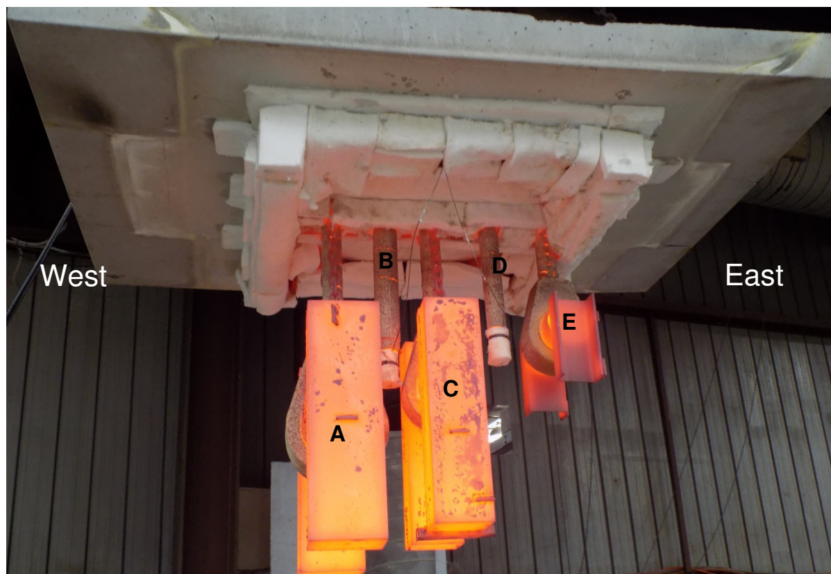
Figure A5.3: Exposed face (side view) of specimen at the end of the test.
