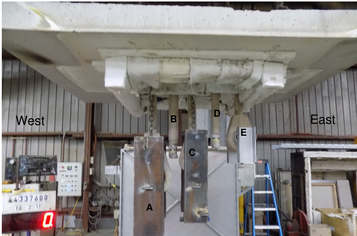
Figure A5.1: Exposed face (side view) of specimen before commencement of the fire-resistance test
